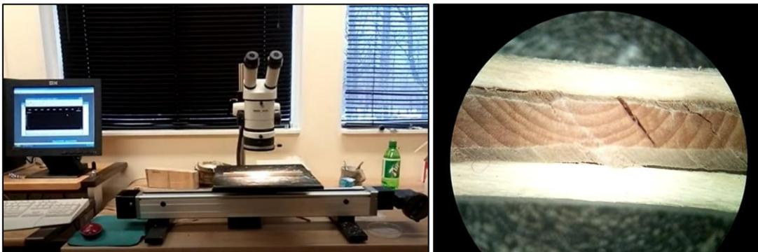
*Figure 9 Rinntech LINTAB measuring apparatus and Rowan Core Sample viewed underneath a Microscope (Hannak 2018)*
