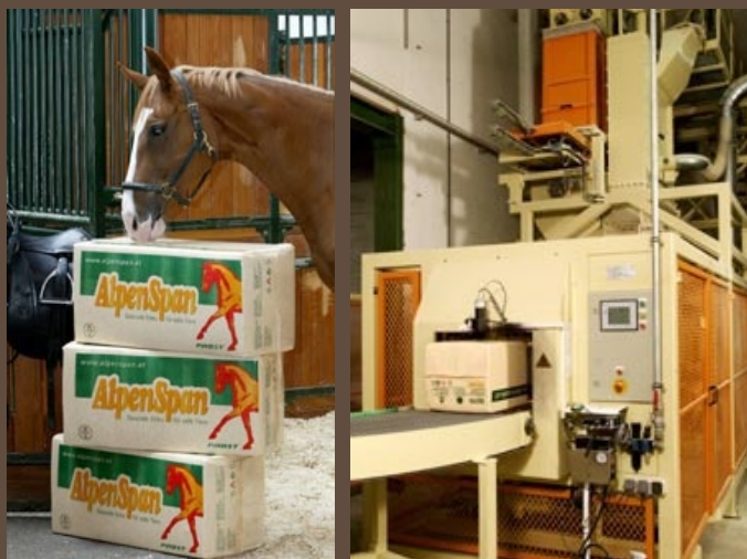
Fig. 1 & 2. AlpenSpan bales and the machine used to shave the wood.
